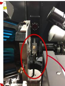
Fig. 2: Sample Setup in Xradia Versa 510.
